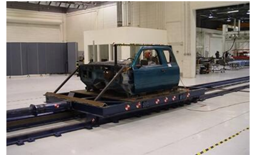
Catapault – Crash Test Sled Repeatable and reliable impact conditions
