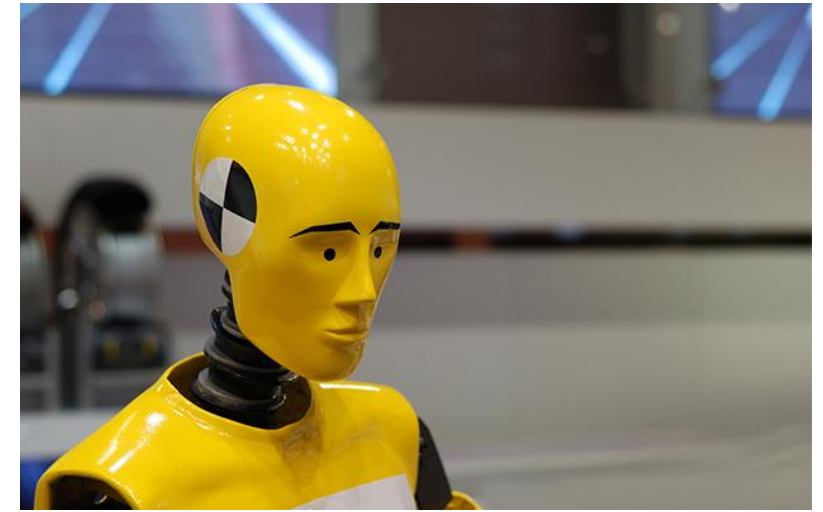
Anthropomorphic Test Device = ATD “Crash Test Dummy”, $200k each
